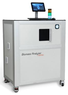
The Biomass Analyzer for determining the quality of wood-based biomass and woodchips.
